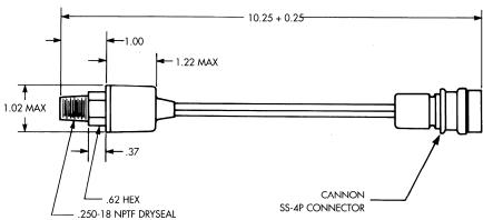
The <u>Model 12000</u> is a diffused silicon based pressure sensor that is ideal for moderate accuracy pressure measurements in industrial and automotive environments.
