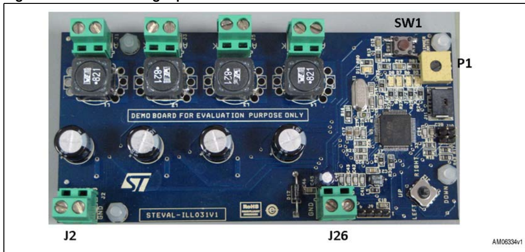
Figure 12. LED street light platform
