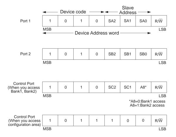
The slave addresses are set as follows when this product is shipped. (SA2, SA1, SA0) = (0, 0, 0) (SB2, SB1, SB0) = (0, 0, 0) (SC2, SC1) = (0, 0)
