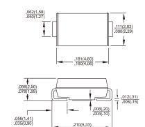
Dimensions in inches and (millimeters) Marking Diagram
