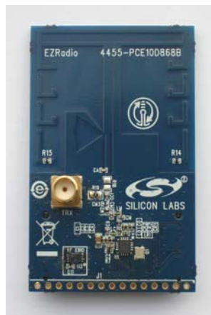
Figure 2. Si4455 RFpico Board—868 MHz (P/N 4455-PCE10D868B)
