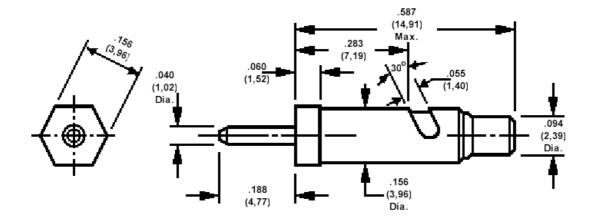
Recommended Lead Wire Sizes - #24 AWG (.020) (0,51) Min. Thru #17 AWG (.045) (1,14) Max.
