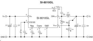
$\begin{array}{cccc} \text{C1: } 220\mu\text{F/63V} & \text{C8: } 0.1\mu\text{F} \\ \text{C2: } 470\mu\text{F/25V} & \text{R1: } 47\Omega \\ \text{C3: } 0.1\mu\text{F} & \text{L1: } 47\mu\text{H} \\ \text{C4: } 1000\text{pF} & \text{D1: RK16} \\ \text{C5: } 0.1\mu\text{F} & (\text{Sanken}) \\ \text{C6: } 0.047\mu\text{F} & \\ \text{C7: } 0.1\mu\text{F} & \end{array}$
