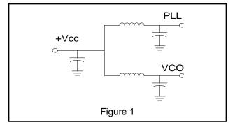
**Note:** Some synthesizers, such as the MASYVS0060-XXXX series, have a single supply pin, and incorporate an on-board regulator and decoupling between the VCO and PLL. This greatly reduces their sensitivity to power supply noise and ripple.
