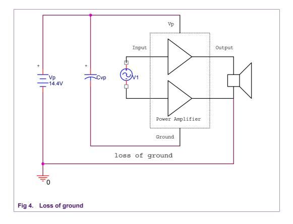
According to figure 4, during a LOG, the peak current which charges the buffer capacitor Cvp, will flow from Cvp into the amplifier ground pin and can destroy the amplifier.
