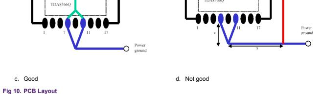
As can be seen in picture 10c is that the signal ground potential of the ground pin (7,11) is equal to the potential of the signal groundconnector of the input signal. In picture 10d the potential between pin 7, 11 and the signal ground connector is unequal, depending on the current-flow through the track, x+y.
