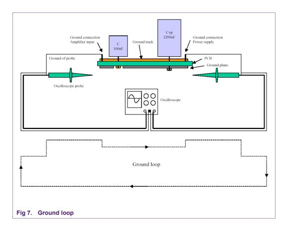
The following drawing shows such a ground loop condition
