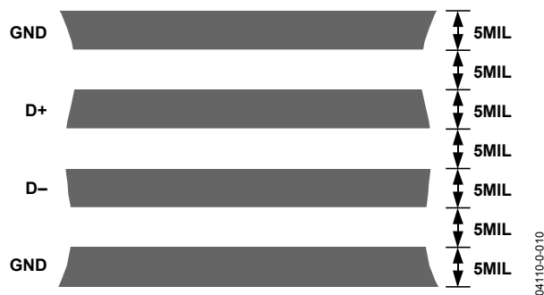
Figure 22. Typical Arrangement of Signal Tracks
