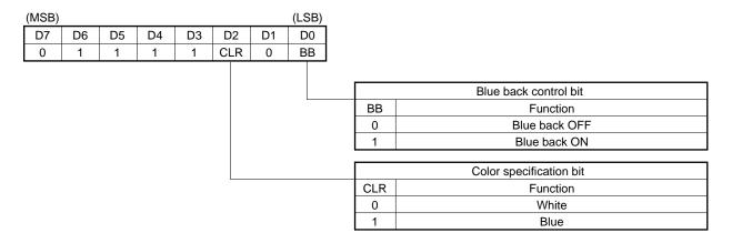
(2) With LSB first (Use of each bit is the same as (1). The command is input from LSB (D0).)
