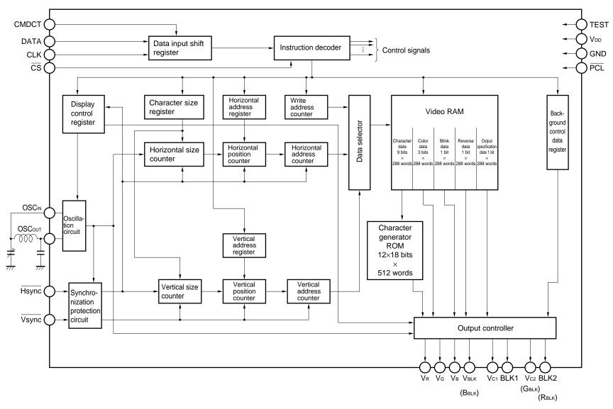
Remark Signals in ( ) are set by using an initial status setting command (RGB + RGB compatible blanking).
