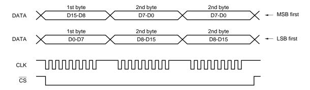
The 2-byte successive command writes characters to the video RAM. To successively write characters without changing the blinking data, reverse specification data, and Vc<sub>2</sub> specification data, first transfer the first byte and then transfer the second byte (character address).
