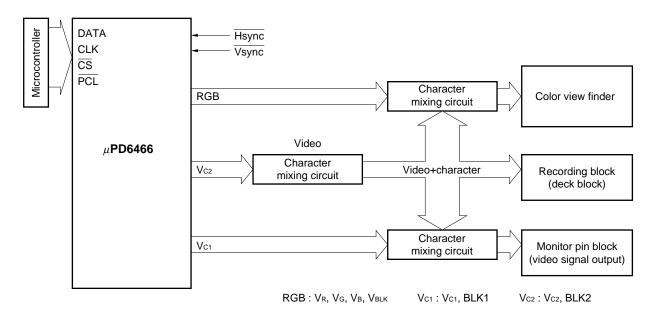
Example of application in a video camera (2) (RGB + 3BLK (RGB compatible BLK)) (When  $V_R$ ,  $V_G$ ,  $V_B$ ,  $R_{BLK}$ ,  $G_{BLK}$ , and  $B_{BLK}$  pins are used)
