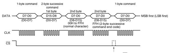
It is not necessary to make  $\overline{\text{CS}}$  low and then back high again.
