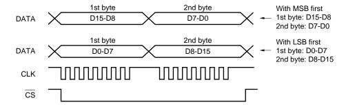
When transferring a 2-byte command, do not make  $\overline{\text{CS}}$  high and keep it low between the first and second bytes.
