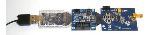
**Note:** Although burning is also possible with this setup, it is not practical since Si4010 is soldered on the key fob development board.
