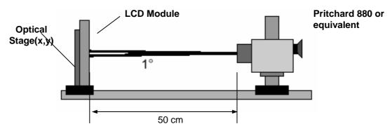
FIG. 1 Optical Characteristic Measurement Equipment and Method
