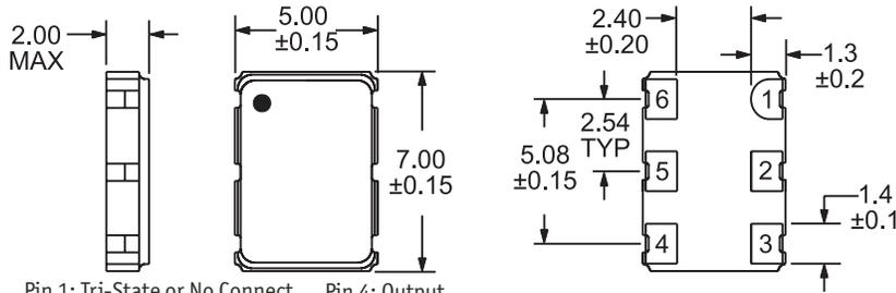
Pin 1: Tri-State or No Connect Pin 4: Output
