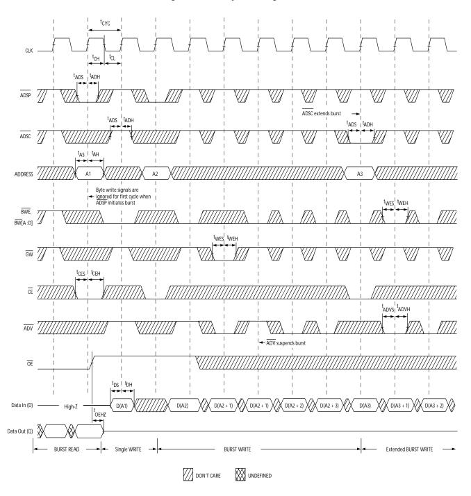
20. On this diagram, when  $\overline{CE}$  is LOW,  $\overline{CE}_1$  is LOW,  $\overline{CE}_2$  is HIGH and  $\overline{CE}_3$  is LOW. When  $\overline{CE}$  is HIGH,  $\overline{CE}_1$  is HIGH or  $\overline{CE}_2$  is LOW or  $\overline{CE}_3$  is HIGH. 21. Full width Write can be initiated by either  $\overline{GW}$  LOW; or by  $\overline{GW}$  HIGH,  $\overline{BWE}$  LOW and  $\overline{BW}_{[A:D]}$  LOW.
