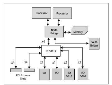
Figure 2 I/O Expansion Application
