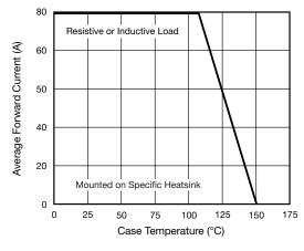
Fig. 1 - Forward Current Derating Curve
