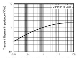
Fig. 6 - Typical Transient Thermal Impedance Per Diode
