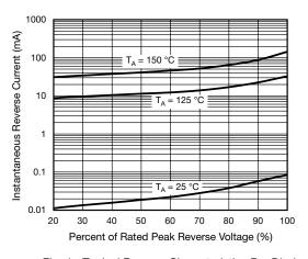
Fig. 4 - Typical Reverse Characteristics Per Diode
