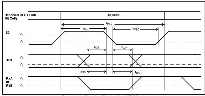
Figure 26 - Receive Timing for CEPT Link
