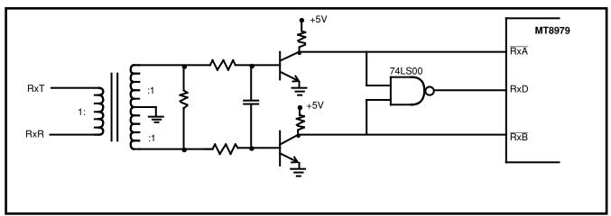
Figure 15 - Typical Bipolar Line Receiver
