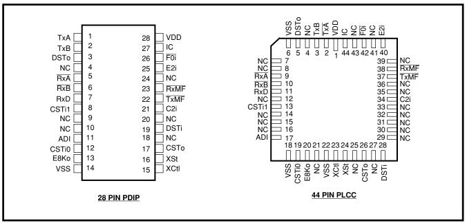
Figure 2 - Pin Connections
