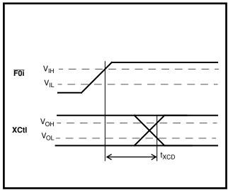
Figure 22 - XCtl Timing
