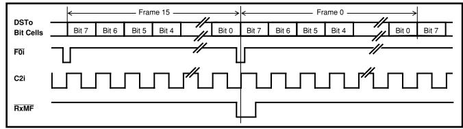
Figure 19 - Functional Timing for Receive Multiframe Clocks
