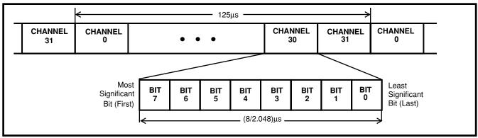
Figure 7 - ST-BUS Stream Format
