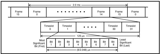
Figure 3 - CEPT Link Frame & Multiframe Format
