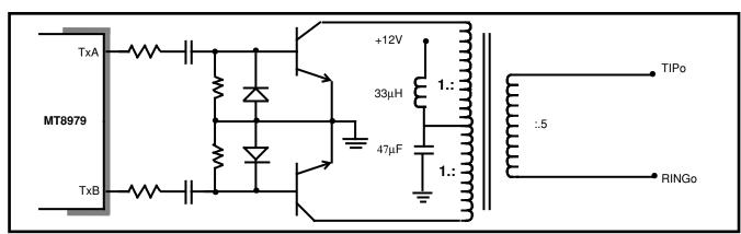
Figure 14 - Bipolar Line Driver
