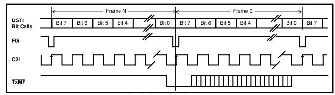
Figure 20 - Functional Timing for Transmit Multiframe Clock
