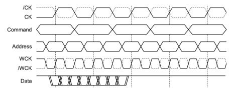
Note: the figure shows the relationship between the data rate of the buses and the clocks and is not a timing diagram.
