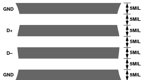
Figure 28. Arrangement of Signal Tracks
