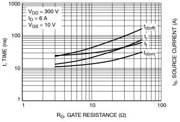
Figure 9. Resistive Switching Time Variation vs. Gate Resistance
