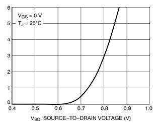
Figure 10. Diode Forward Voltage vs. Current
