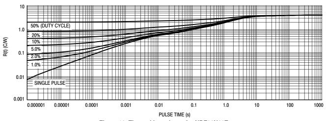
Figure 12. Thermal Impedance for NDF06N60Z
