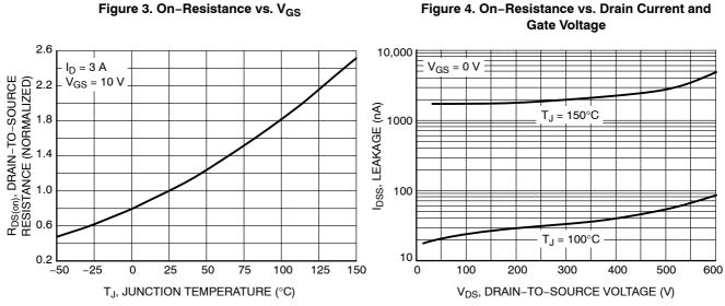
Figure 5. On-Resistance Variation with **Temperature** www.DataSheet4U.com
