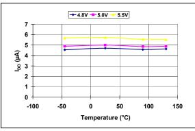
FIGURE 2-7: I<sub>DD</sub> vs. Temperature (Watchdog Timer Active) (MCP1318M-4.6).
