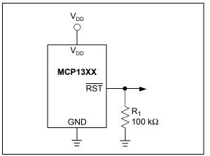
**FIGURE 5-8:** Ensuring a valid active-low Reset pin output state as V<sub>DD</sub> approaches 0V.
