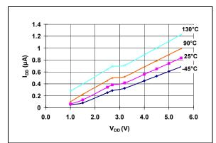
**FIGURE 2-11:** I<sub>DD</sub> vs. V<sub>DD</sub> (Reset Power-up Timer Inactive and Watchdog Timer Inactive) (**MCP1319-2.9**).
