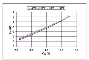
**FIGURE 2-15:** I<sub>DD</sub> vs. V<sub>DD</sub> (Reset Power-up Timer Active or Watchdog Timer Active) (**MCP1316-2.0**).
