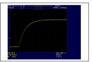
FIGURE 2-49: "M" Part # Pull-up Characteristics (MCP1318M-4.6).
