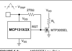
FIGURE 5-6: MOSFET Low-Drive Protection.
