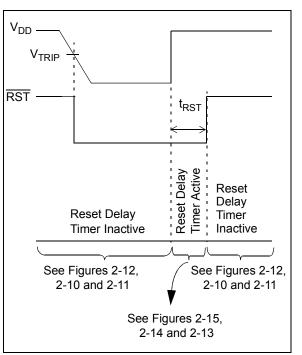
FIGURE 4-15: Reset Power-up Timer Waveform.
