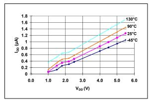
**FIGURE 2-12:** I<sub>DD</sub> vs. V<sub>DD</sub> (Reset Power-up Timer Inactive and Watchdog Timer Inactive) (**MCP1316-2.0**).
