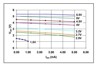
FIGURE 2-26: V<sub>OH</sub> vs. I<sub>OH</sub> (MCP1319-2.9 @ 25C).
