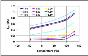
**FIGURE 2-1:** I<sub>DD</sub> vs. Temperature (Reset Power-up Timer Inactive and Watchdog Timer Inactive) (**MCP1318M-4.6**).
