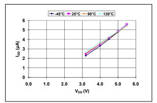
**FIGURE 2-14:** I<sub>DD</sub> vs. V<sub>DD</sub> (Reset Power-up Timer Active or Watchdog Timer Active) (**MCP1319-2.9**).
