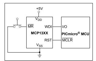
FIGURE 4-17: Push Button Reset and Watchdog Timer.
