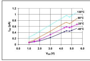
**FIGURE 2-10:** I<sub>DD</sub> vs. V<sub>DD</sub> (Reset Power-up Timer Inactive and Watchdog Timer Inactive) (**MCP1318M-4.6**).
