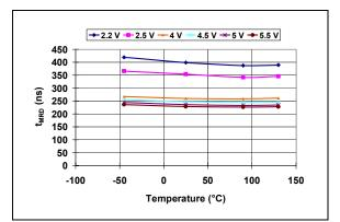
FIGURE 2-38: MR Low to Reset Propagation Delay (MCP1316-2.0).
