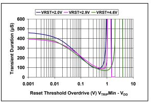
**FIGURE 2-48:** Max V<sub>DD</sub> Transient Duration vs. Reset Threshold Overdrive.
