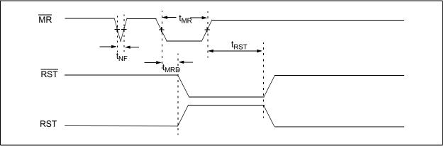
FIGURE 1-2: MR and Reset Pin Waveforms.
