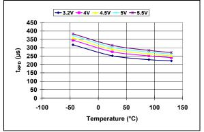
*FIGURE 2-29: t<sub>RPD</sub> vs. Temperature* (*MCP1319-2.9*).
