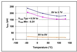
**FIGURE 2-40:** V<sub>DD</sub> Falling to Reset Propagation Delay vs. Temperature (**MCP1319-2.9**).
