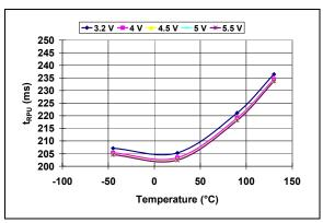
*FIGURE 2-32: t<sub>RPU</sub> vs. Temperature* (*MCP1319-2.9*).
