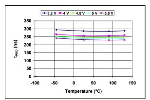
FIGURE 2-37: MR Low to Reset Propagation Delay (MCP1319-2.9).
