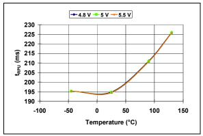
*FIGURE 2-31: t<sub>RPU</sub> vs. Temperature* (*MCP1318M-4.6*).
