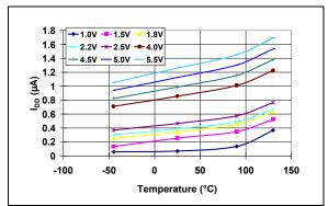
**FIGURE 2-3:** I<sub>DD</sub> vs. Temperature (Reset Power-up Timer Inactive and Watchdog Timer Inactive) (**MCP1316-2.0**).
