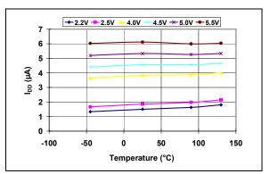
**FIGURE 2-6:** I<sub>DD</sub> vs. Temperature (Reset Power-up Timer Active) (**MCP1316-2.0**).
