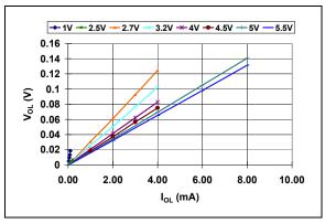
**FIGURE 2-20:** V<sub>OL</sub> vs. I<sub>OL</sub> (MCP1319-2.9).
