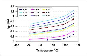
**FIGURE 2-2:** I<sub>DD</sub> vs. Temperature (Reset Power-up Timer Inactive and Watchdog Timer Inactive) (**MCP1319-2.9**).
