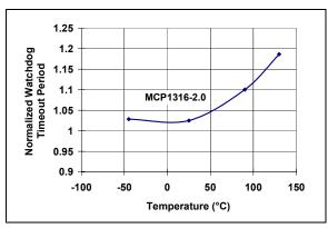
FIGURE 2-47: Normalized Watchdog Time Out Period vs. Temperature (MCP1316-2.0).
