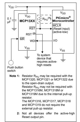
FIGURE 4-1: Typical Application Circuit.
