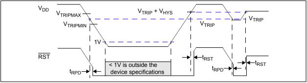
**FIGURE 4-14:** RST Operation as determined by the  $V_{TRIP}$  and  $V_{HYS}$ .
