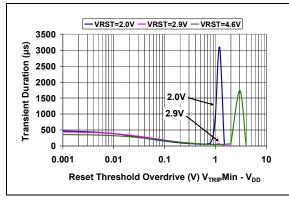
**FIGURE 2-34:** Transient Duration vs.  $V_{TRIP}$  (min) –  $V_{DD}$ .
