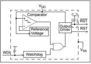
FIGURE 4-7: MCP1318M Block Diagram.
