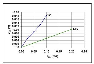
FIGURE 2-21: V<sub>OL</sub> vs. I<sub>OL</sub> (MCP1316-2.0).
