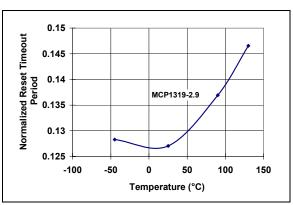
FIGURE 2-43: Normalized Reset Time Out Period vs. Temperature (MCP1319-2.9).
