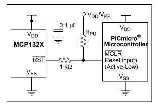
**FIGURE 5-4:** Typical Application Circuit for PICmicro<sup>®</sup> Microcontroller with the ICSP™ Feature.
