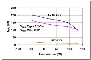
**FIGURE 2-41:** V<sub>DD</sub> Falling to Reset Propagation Delay vs. Temperature (**MCP1316-2.0**).
