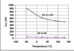
**FIGURE 2-39:** V<sub>DD</sub> Falling to Reset Propagation Delay vs. Temperature (**MCP1318M-4.6**).
