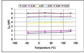
FIGURE 2-9: I<sub>DD</sub> vs. Temperature (Watchdog Timer Active) (MCP1316-2.0).
