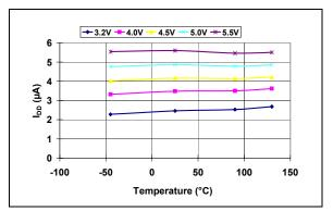
*FIGURE 2-5: I*<sub>DD</sub> vs. Temperature (Reset Power-up Timer Active) (**MCP1319-2.9**).
