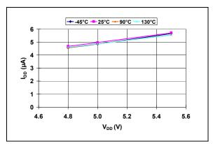
**FIGURE 2-13:** I<sub>DD</sub> vs. V<sub>DD</sub> (Reset Power-up Timer Active or Watchdog Timer Active) (**MCP1318M-4.6**).
