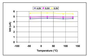
**FIGURE 2-4:** I<sub>DD</sub> vs. Temperature (Reset Power-up Timer Active) (**MCP1318M-4.6**).
