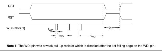
FIGURE 1-3: WDI and Reset Pin Waveforms.
