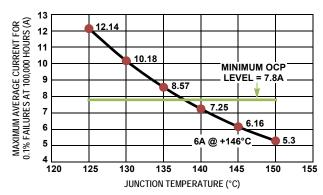
FIGURE 10. CURRENT vs TEMPERATURE
