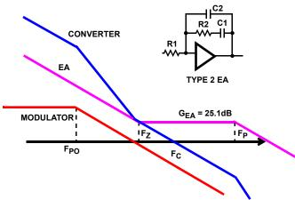
FIGURE 9. FEEDBACK LOOP COMPENSATION
