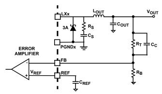
FIGURE 11. SCHOTTKY DIODE AND R-C SNUBBER
