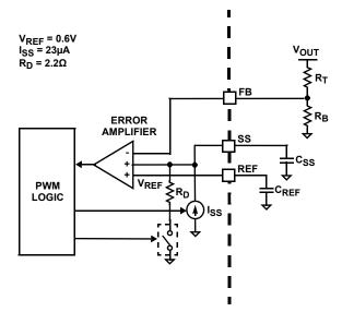
FIGURE 8. SOFT-START CIRCUIT
