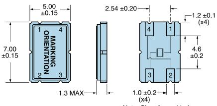
Note: Chamfer and index mark not shown.
