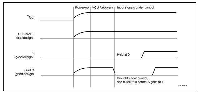
While the Chip Select (S) input is held Low, the chip is not selected, and it does not matter what signals occur on the other lines (provided that they remain within the specified safe range). It is only necessary, therefore, for the Chip Select (S) input to be tied Low by a pull-down resistor, as shown in Figure 5, so that it never goes High when it is undriven, as confirmed in Figure 4.
