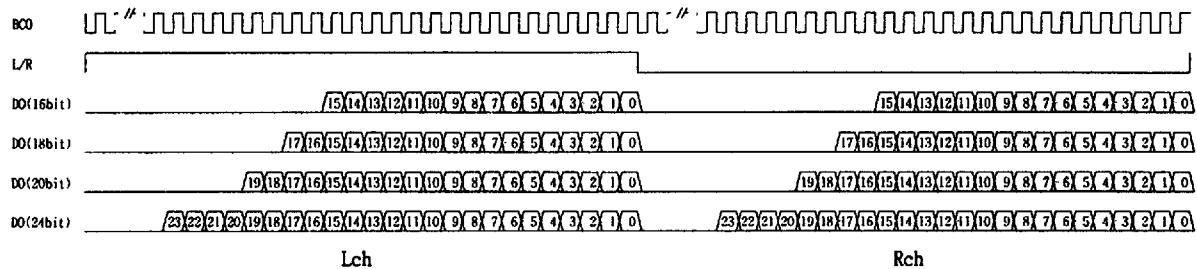
4-3) The digital audio interface is made compatible with the following format with OPR register (\$00) and DAR register (\$04).
