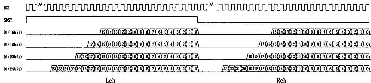
4-2) Digital audio signal is outputted through BCO, L/R, and DO pins using the following format.
