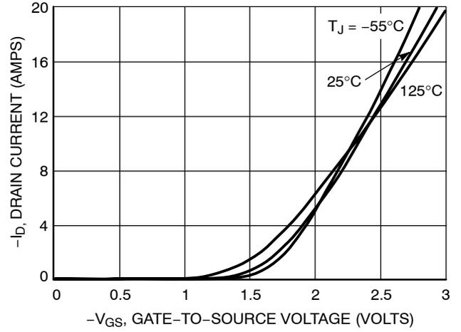
Figure 2. Transfer Characteristics
