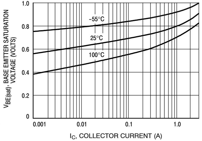
**Figure 13. Base Emitter Saturation Voltage versus Collector Current**
