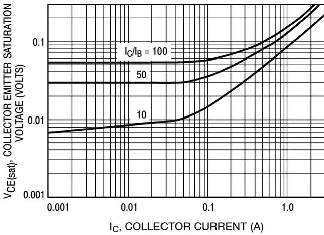
**Figure 10. Collector Emitter Saturation Voltage versus Collector Current**
