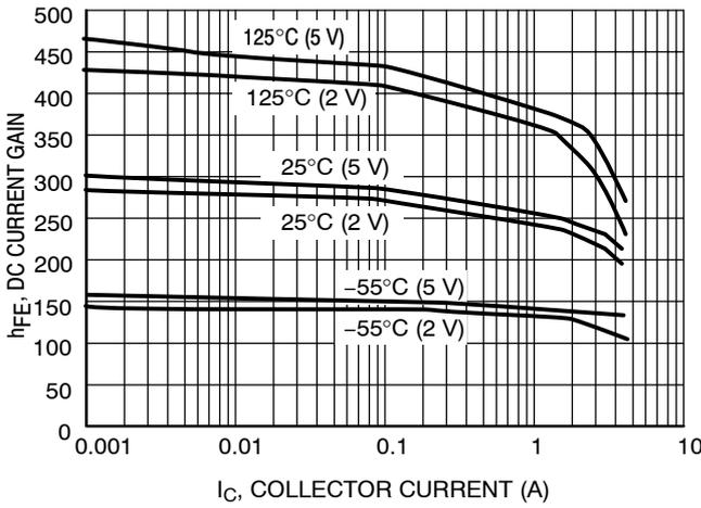
**Figure 12. DC Current Gain versus Collector Current**
