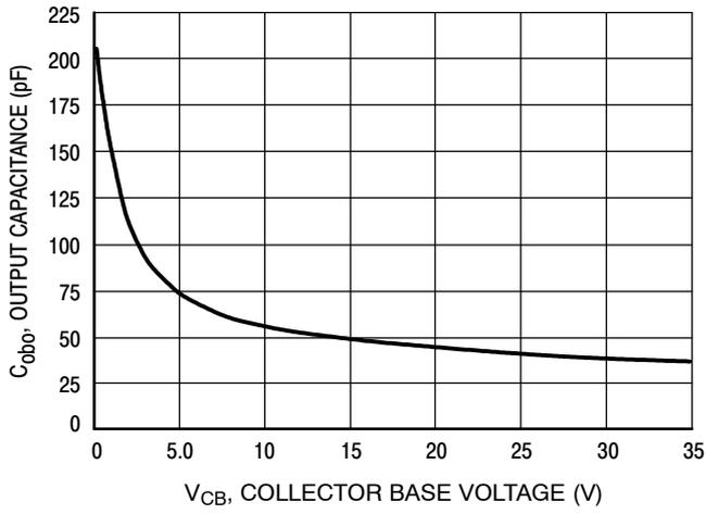
Figure 16. Output Capacitance
