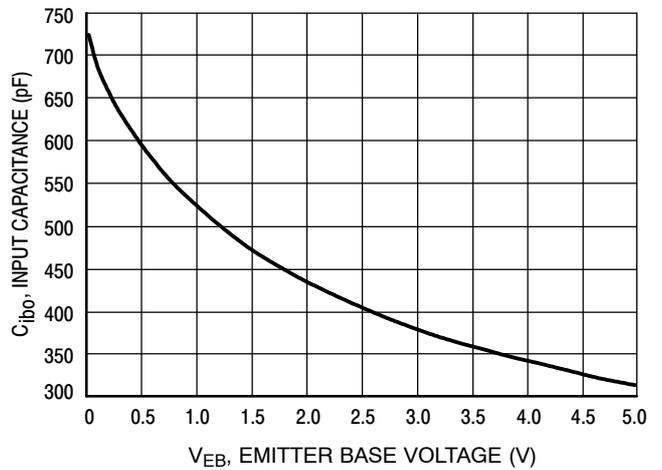
**Figure 15. Input Capacitance**
