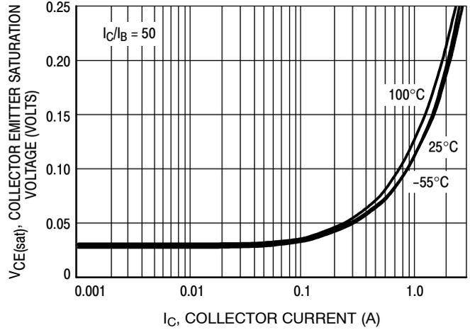
**Figure 11. Collector Emitter Saturation Voltage versus Collector Current**
