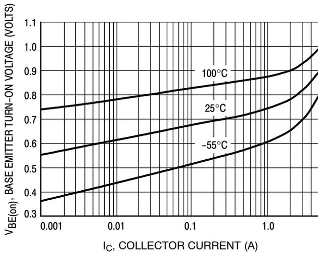
**Figure 14. Base Emitter Turn-On Voltage versus Collector Current**
