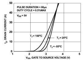
Figure 5. Transfer Characteristics
