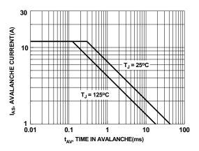
Figure 9. Unclamped Inductive Switching Capability
