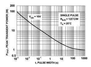
Figure 12. Single Pulse Maximum Power Dissipation
