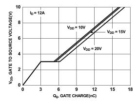
Figure 7. Gate Charge Characteristics
