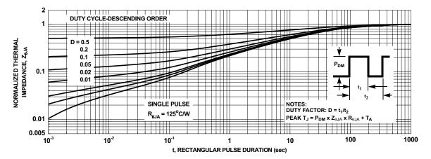
Figure 13. Transient Thermal Response Curve
