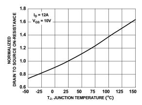
Figure 3. Normalized On-Resistance vs Junction Temperature
