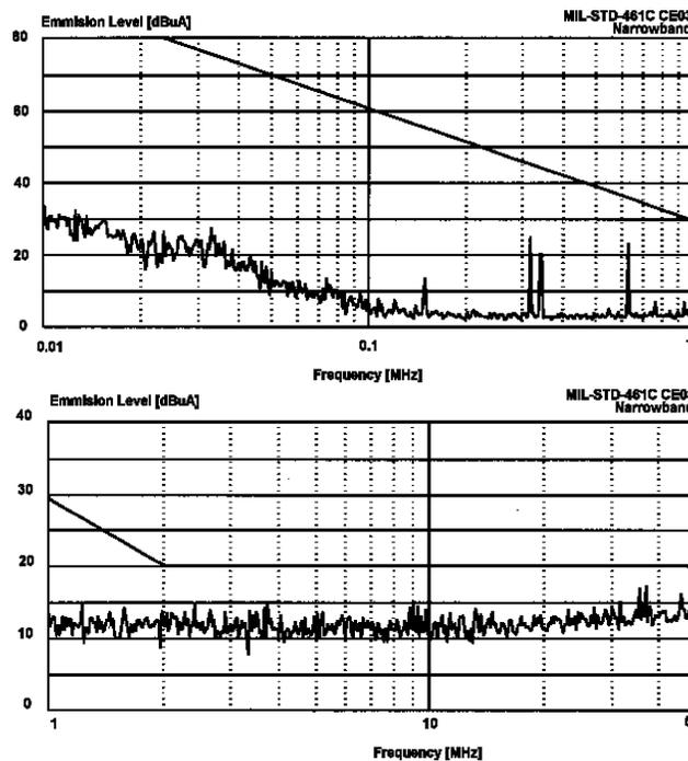
**Figure 10 – DVHF+2800T with EMI Filter**
