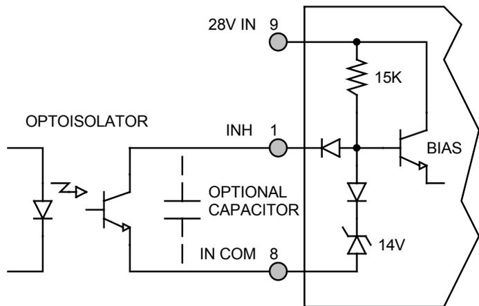
**Figure 5 – Isolated Inhibit Drive**
