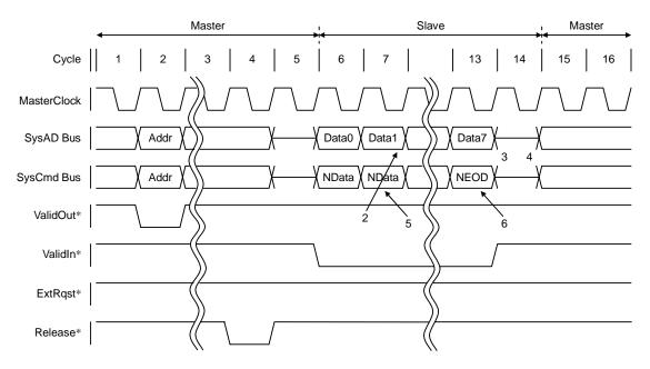
Figure 11.2.23 Block Read Response when System Interface is in the Slave State
