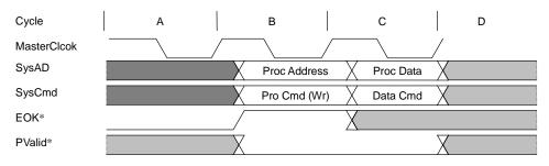
Figure 11.3.9 Sample Cycle with EOK\* Asserted, Then Deasserted
