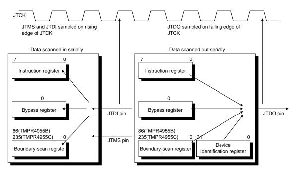
Figure 14.3.7 JTAG Test Access Port
