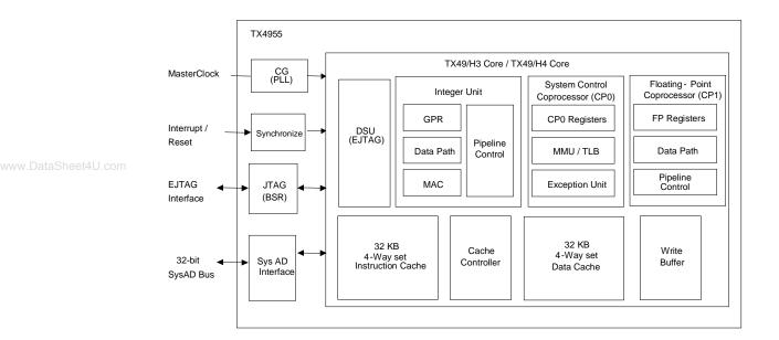
Figure 2.1.1 TX4955 Block Diagram
