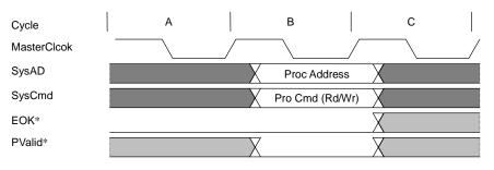
Figure 11.3.8 Sample Cycle with EOK\* Asserted
