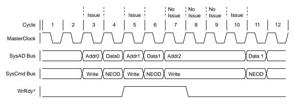
Figure 11.2.16 Pipeline Write Protocol
