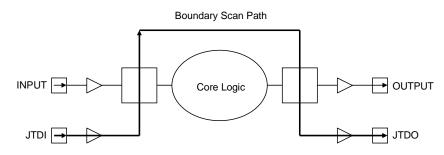
Figure 14.4.3 Test Data Flow While PRELOAD is Selected
