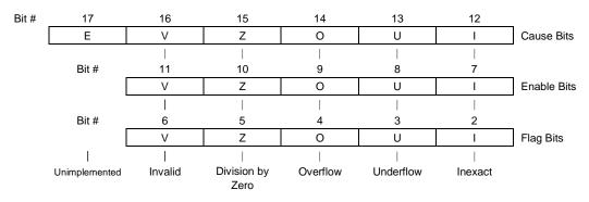
Figure 8.21.1 Control/Status Register (Exception/Flag/Trap/Enable Bits)
