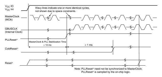
Figure 9.2.1 Power-On Reset Timing
