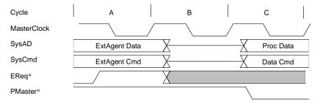
Figure 11.3.11 Sample Cycle with Deassertion of EReq\*
