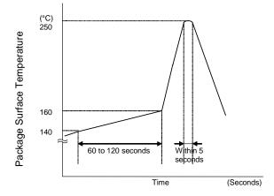
Figure 3.5 Example of Surface-Mount Package Temperature Profile
