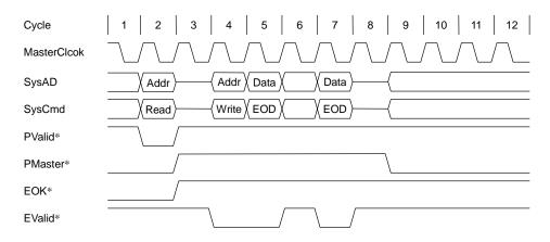
Figure 11.3.21 External Write Followed By External Read Response, System Interface In Slave State
