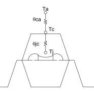
Figure 3.2 Thermal Resistance of Package
