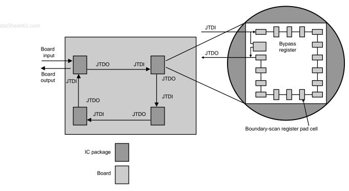
Figure 14.3.3 Bypass Register Operation
