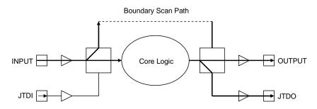
Figure 14.4.2 Test Data Flow While SAMPLE is Selected
