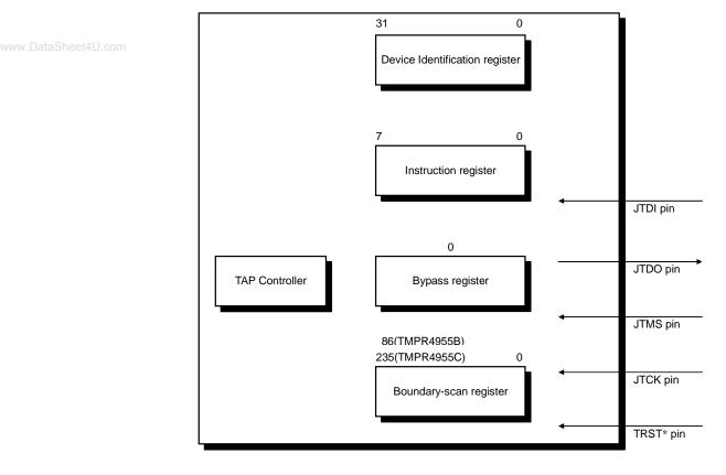
Figure 14.2.1 JTAG Interface Signals and Registers
