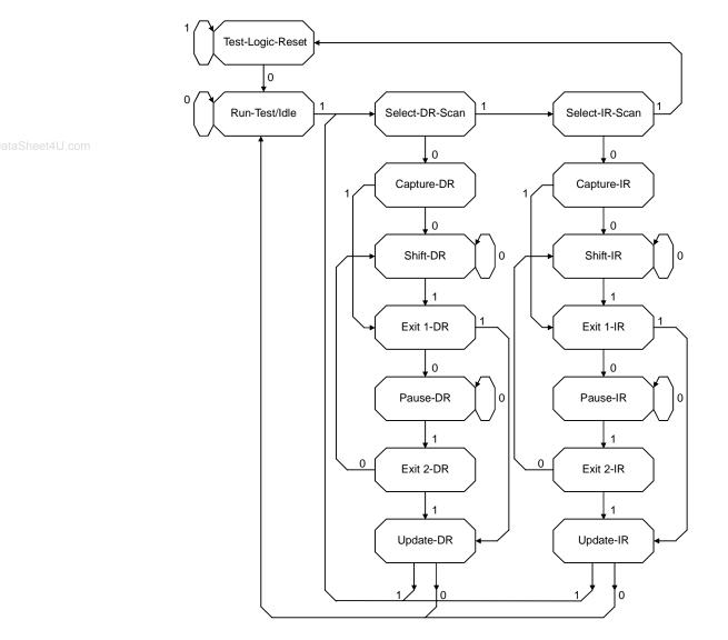
Figure 14.3.8 TAP Controller State Diagram
