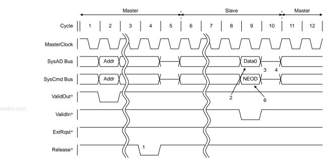
Figure 11.2.22 Processor Word Read Request and Subsequent Word Read Response
