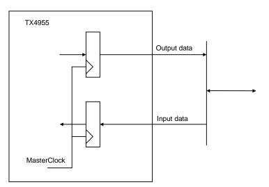
Figure 11.3.2 System Interface Register-to-Register Operation
