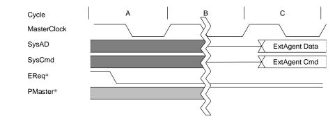
Figure 11.3.10 Sample Cycle with EReq\* Asserted
