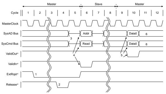
Figure 11.2.19 External Read Request when System Interface is in the Master State
