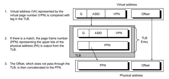
Figure 4.1.1 Overview of a Virtual-to-Physical Address Translation
