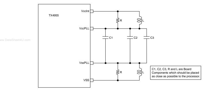
Figure A.1 PLL Recommended Circuit
