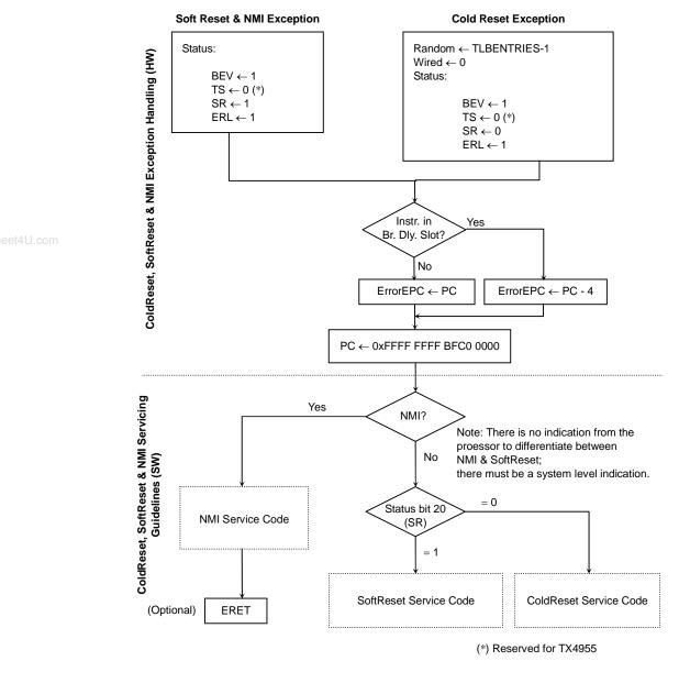
Figure 8.20.5 ColdReset, SoftReset & NMI Exception Handling (HW) and
