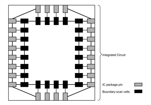
Figure 14.1.1 JTAG Boundary-scan Cells
