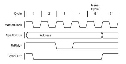
Figure 11.2.2 RdRdy\* Signal Status in case of Read Request
