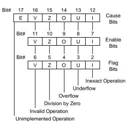
Figure 3.3.4 Control/Status Register Cause, Flag, and Enable Fields
