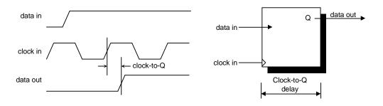
Figure 10.1.2 Clock-to-Q Delay
