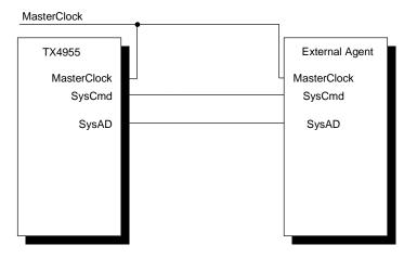
Figure 10.3.1 The TX4955 Processor Phase-Locked System
