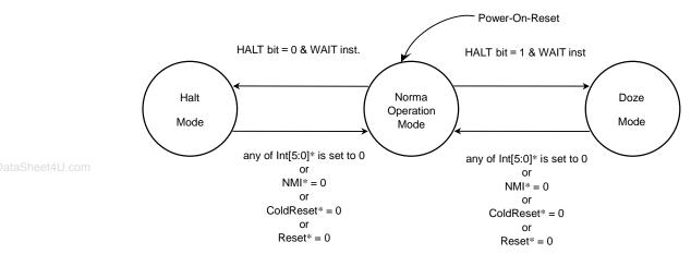
Figure 13.3.1 shows the status shifts in the operation mode of the TX4955.
