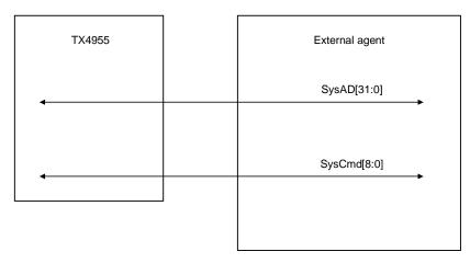
Figure 11.2.1 System Interface Bus
