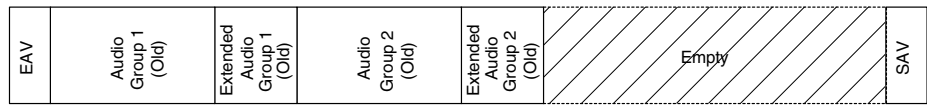
Video signal after GS9023B Removal of Audio Group 1 & Extended Audio Group 1 (ANCI = LOW or "VSEL" = HIGH and "ADEL" = LOW)
