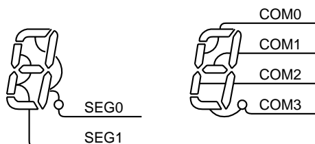
Figure 13-6 Example of COM, SEG Pin Connection (1/4 Duty)
