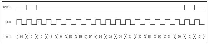
Figure 17. DSP Interface—Continuous Conversion
