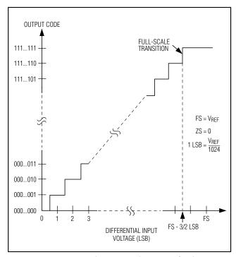
Figure 8. Unipolar Transfer Function (MAX1072 Only)
