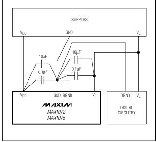
Figure 20. Power-Supply Grounding Condition
