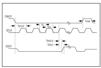
Figure 1. Detailed Serial-Interface Timing
