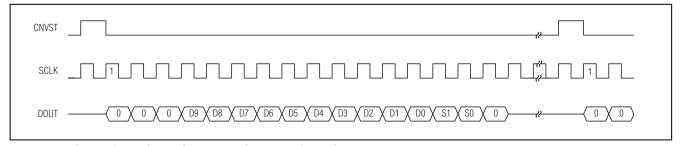
Figure 18. DSP Interface—Single-Conversion, Continuous/Burst Clock
