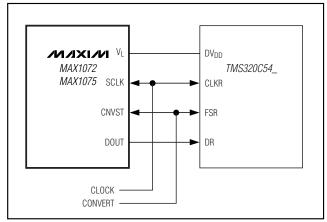
Figure 16. Interfacing to the TMS320C54\_ External Clocks
