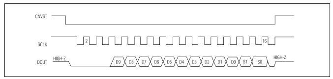
Figure 14. QSPI Serial-Interface Timing—Single Conversion (CPOL = 1, CPHA = 1)
