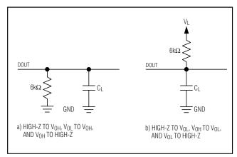
Figure 2. Load Circuits for Enable/Disable Times
