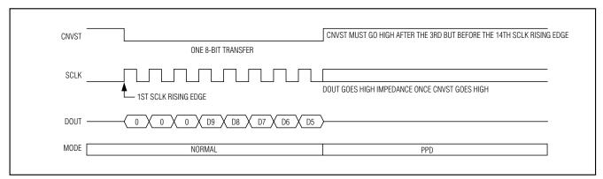
Figure 6. SPI Interface—Partial Power-Down Mode
