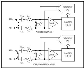
Figure 4. Equivalent Input Circuit
