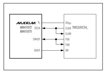
Figure 15. Interfacing to the TMS320C54\_ Internal Clocks
