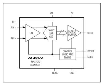
Figure 3. Functional Diagram
