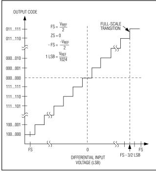
Figure 9. Bipolar Transfer Function (MAX1075 Only)
