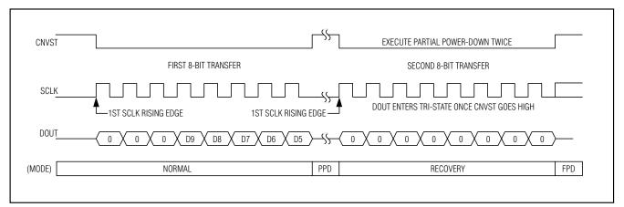
Figure 7. SPI Interface—Full Power-Down Mode
