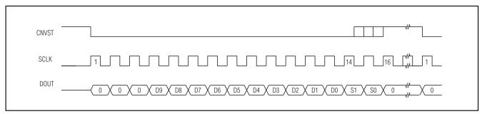
Figure 10. Continuous Conversion with Burst/Continuous Clock
