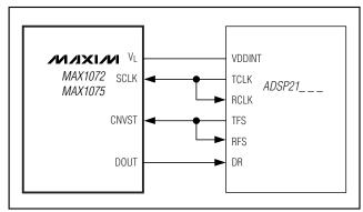
Figure 19. Interfacing to the ADSP21\_ \_ \_
