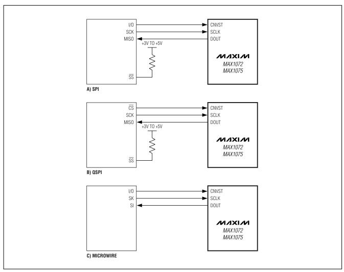
Figure 11. Common Serial-Interface Connections to the MAX1072/MAX1075
