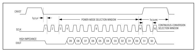
Figure 5. Interface-Timing Sequence
