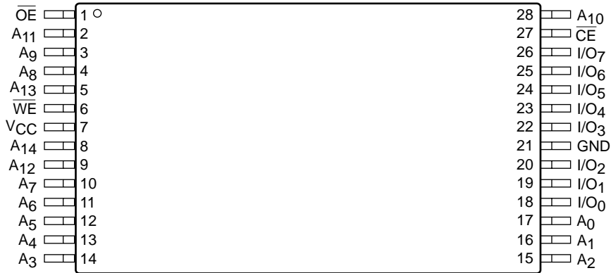
TSOP Top View (8mm X 13.4mm) (H13)
