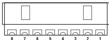
Figure 2. Rear view diagram with pinout.
