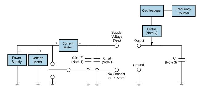
Note 1: An external  $0.1\mu\text{F}$  low frequency tantalum bypass capacitor in parallel with a  $0.01\mu\text{F}$  high frequency ceramic bypass capacitor close to the package ground and  $V_{DD}$  pin is required.
