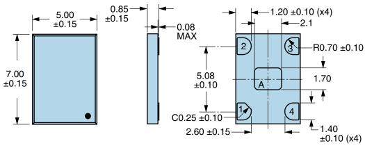
PIN CONNECTION Tri-State (High 1 Impedance) Ground 2 3 Output 4 Supply Voltage LINE MARKING XXXX or XXXXX XXXX or XXXXX=Ecliptek 1 Manufacturing Lot Code
