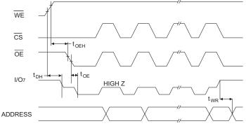
**TOGGLE BIT:** In addition to DATA Polling another method for determining the end of a write cycle is provided . During the write operation, successive attempts to read data from the device will result in I/O<sub>6</sub> toggling between one and zero. Once the write has completed, I/O<sub>6</sub> will stop toggling and valid data will be read. Reading the toggle bit may begin at any time during the write cycle. Toggle But Characteristics<sup>(1)</sup>
