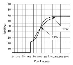
FIG.1 The relation curve between f<sub>SW</sub> and relative output power P<sub>OUT</sub>/ P<sub>OUT (MAX)</sub>
