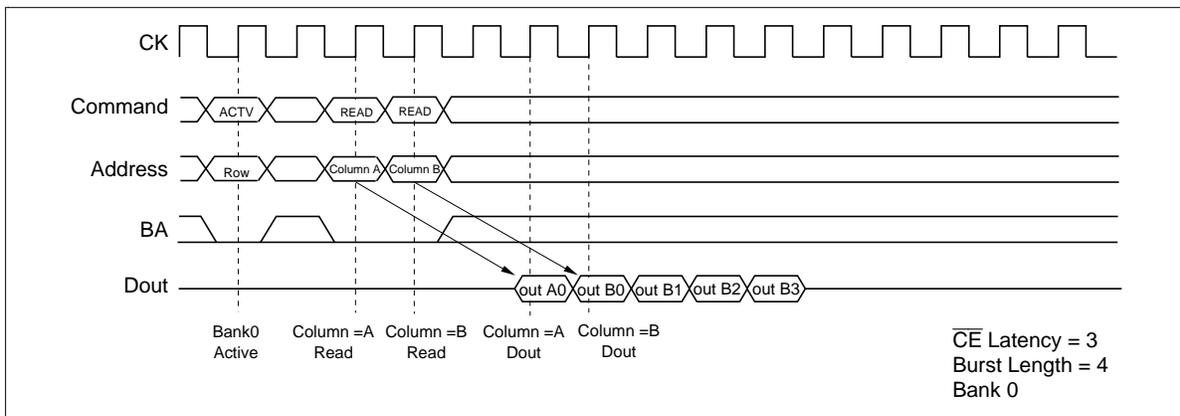
**2. Same bank, different ROW address:** When the ROW address changes on same bank, consecutive read commands cannot be executed; it is necessary to separate the two read commands with a precharge command and a bank-active command.
