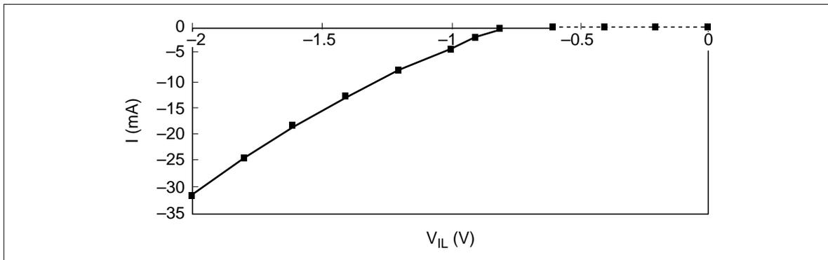
**Minimum  $V_{IH}$  Clamp Current**
