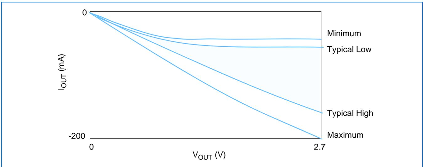
5. The full variation in the ratio of the maximum to minimum pullup and pulldown current will not exceed 1.7, for device drain to source voltages from 0.1 to 1.0.
