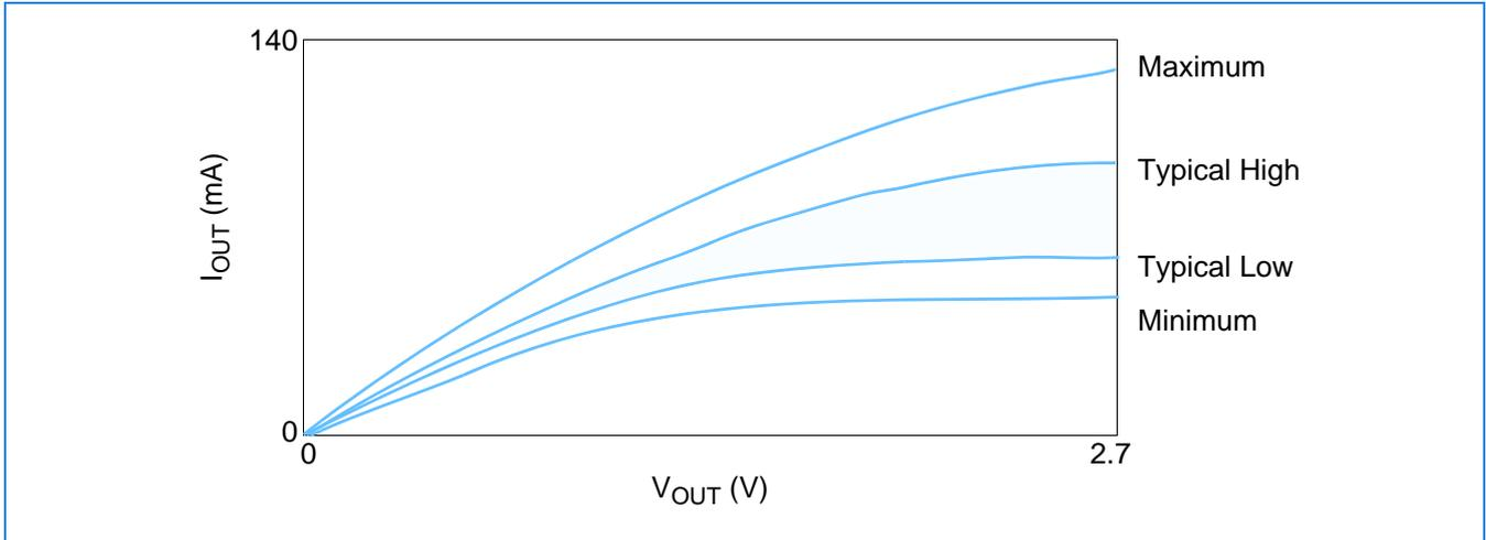
3. The full variation in driver pullup current from minimum to maximum process, temperature and voltage will lie within the outer bounding lines of the V-I curve.
