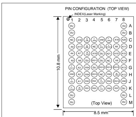
F-VCC : VCC for Flash F-RP# : Reset power down for Flash M-VCC : VCC for Mobile RAM F-WP# : Write protect for Flash **GND** : GND for Flash / Mobile RAM F-RY/BY# : Flash Memory Ready /Busy A0-A21 : Common address for Flash/Mobile RAM M-CE# : Mobile RAM chip enable DQ0-DQ15: Data I/O M-OE# : Output enable for Mobile RAM
