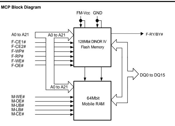
Note: In the 128M-bit DINOR(IV) Flash Memory lower 64Mbit is selected by F-CE1#="L" and upper 64Mbit is done by F-CE2#="L". Never select each chip at the same time. In the data sheet there are "VCC"s which mean "FM-VCC" (Common Vcc for Flash / Mobile RAM). In the Flash Memory part they mean OE# and WE# are F-OE# and F-WE#.
