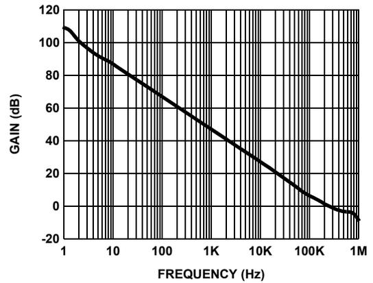
FIGURE 8.  $A_{VOL}$  vs FREQUENCY @ 100k $\Omega$  LOAD
