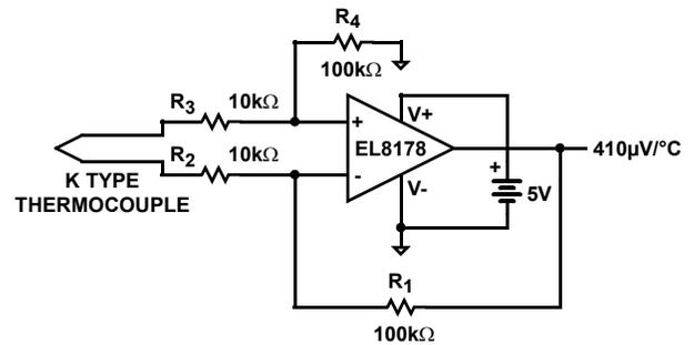
FIGURE 12. THERMOCOUPLE AMPLIFIER
