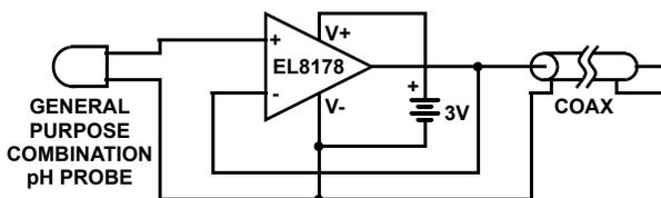
FIGURE 11. PH PROBE AMPLIFIER
