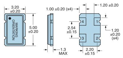
Note: Pin 1 Chamfer not shown.
