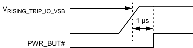
Figure 7-12. Skip Electrical Parameters
