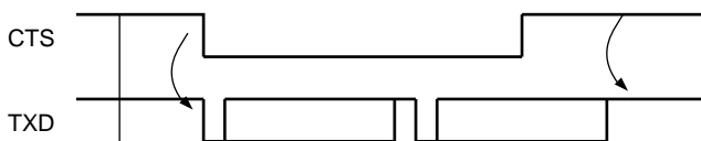
Figure 25-28. Transmitter Behavior when Operating with Hardware Handshaking
