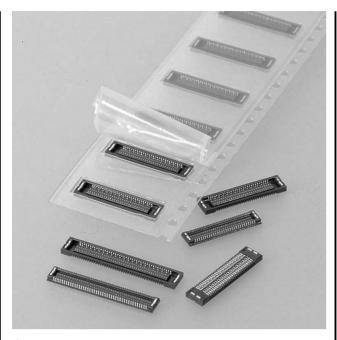
SMT configuration 0.4mm pitch board-toboard connector with 4-row staggered leads that are located just below the surface of the wafer. With the CSP (chip size package) technology, mounting area on the board is minimized.
