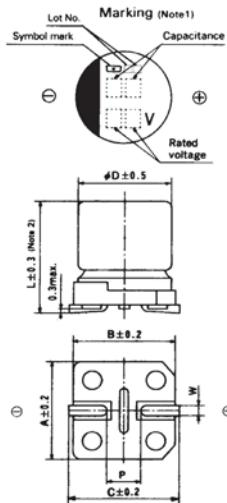
Note 1 : For case size 8x10(H10) and 10X10(J10).the pvc sleeve with marking covers the side of the body.
