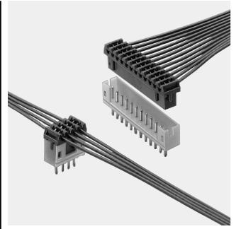
This 2.0mm (.079") pitch insulation displacement connector is another version of the NRD connector for printed circuit boards. The KRD connector allows daisy chaining and is very useful in simplifying connection systems in electronic equipment.
